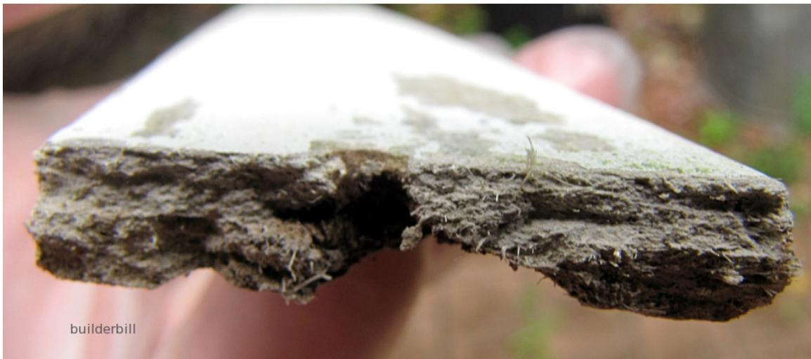
Img 5.3: A close up of the end of a broken batten showing clumps of loose fibres.
