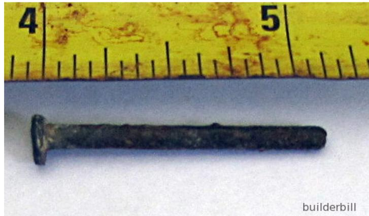
Img 5.4: A typical 30 x 2.8 shear point galvanized Fibro nail.
