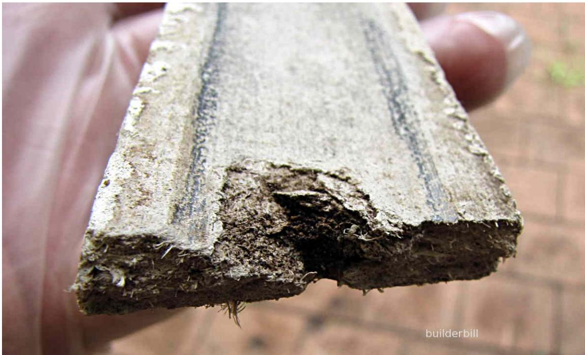
Img 5.7: The back side of an AC batten is recessed by about 3mm. This shows typical breaking away of material on the inside edge at the nail point.
